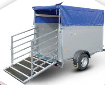
VZ O with a ramp and side railing
