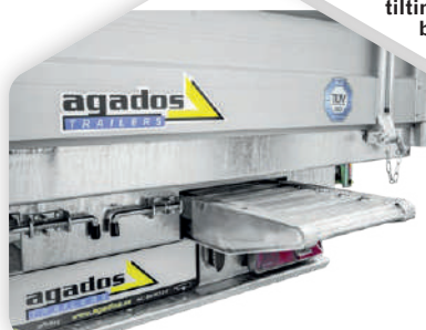
Detail of ramp lodgement under the loading area
