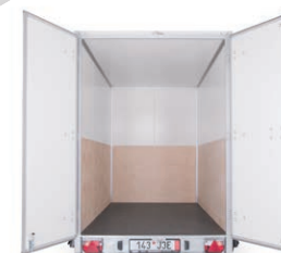
VZ 31 B2, 2000 kg with protective inner lining
