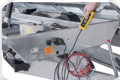
Hydraulic three-sided tilting of the body
