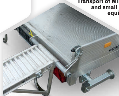
Ramps with supports, sliding aside according to the wheel track of the transport machine
