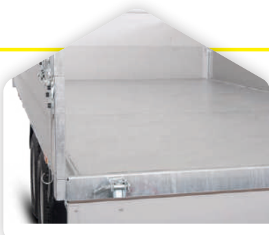
Waterproof plywood floor covered with Zn metal sheet
