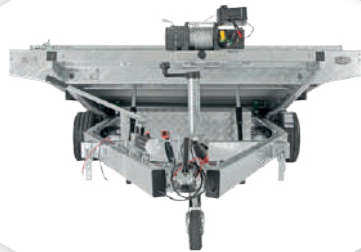
Sliding winch across the entire width of the trailer
