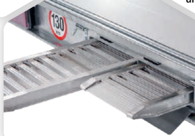
Ramp lodgement un- der the loading area
