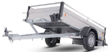
ALUX in tilting design with a hand jack
