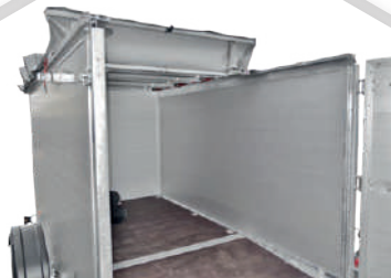
Detail – box design with folding roof
