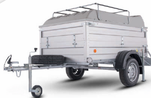
VZ with aluminium side boards, side board superstructure and lockable plastic cover
