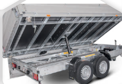
Three-sided tilting – detail
